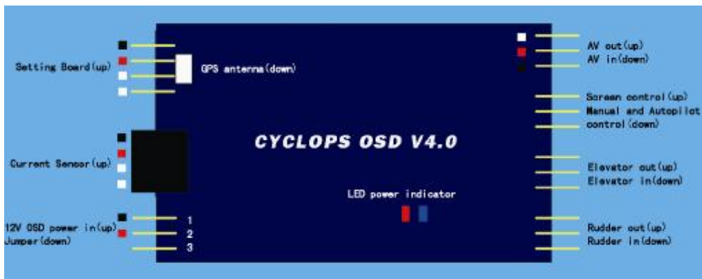
Current sensor connection diagram
